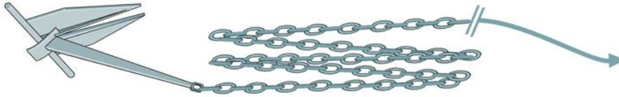
Figure 3. Laying the anchor chain and rope on the deck ready to deploy, anchor end first.
